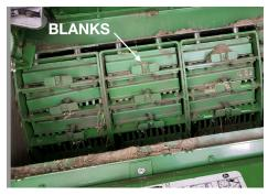
If the chaffer is being overloaded on a particular side then **ADD 2-3 BLANKS to the top of the separation grates (as seen above) to the side overloading**. With a stripper header, you will likely want to run blanks as well.
